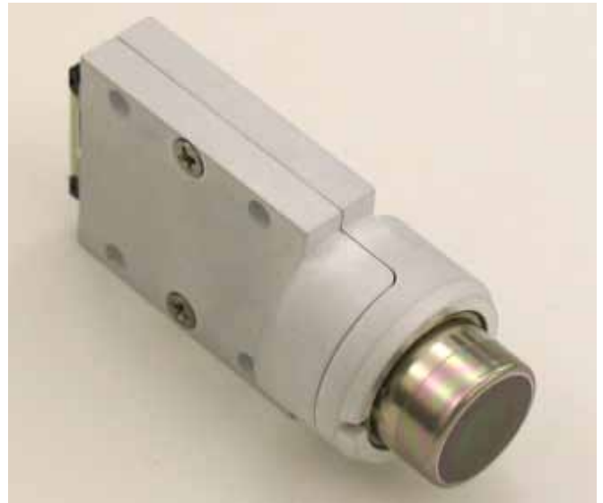
Figure 9. PA-210 Housing. The PA-210 can be ordered with a housing that completely shields the detector and preamplifier and provides heat-sinking and mounting holes. This optional housing saves the OEM the design time of fabricating a custom enclosure.
