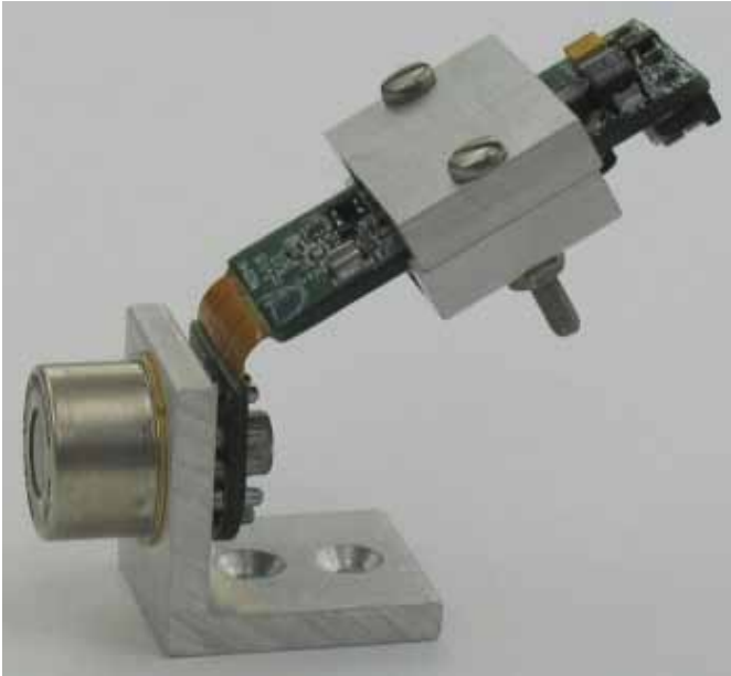
Figure 12. PA230 flexible preamplifier with detector, heat-sink, and mounting hardware.
