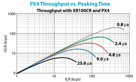
PX4 throughput for various peaking times. Taken with an Amptek XR100CR X-Ray Detector.
